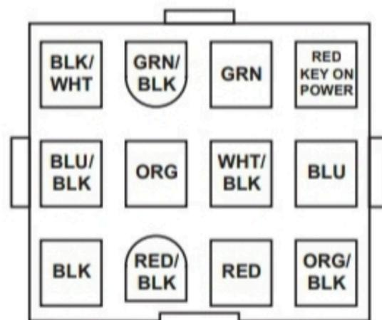
**Connector Body - Cab side SP-C11 Truck Control Wire**
